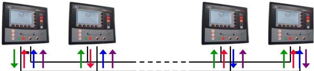
FIGURE 85 - TRANSMISSION DE DONNÉES ENTRE MODULES
