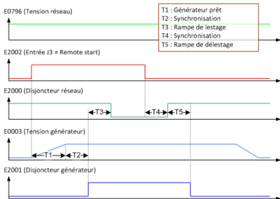
FIGURE 27 - SÉQUENCE TYPE EN MODE FUGITIF SUR DÉMARRAGE EXTERNE
