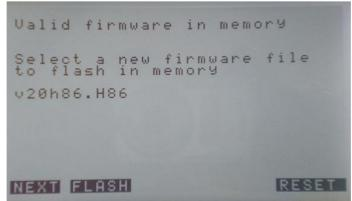
"**NEXT**" button allows you to select the required H86 file (if several H86 files are present on the SD card). "**FLASH**" button allows you to start the flashing. While upgrading firmware, the number of processed bytes will increase.
