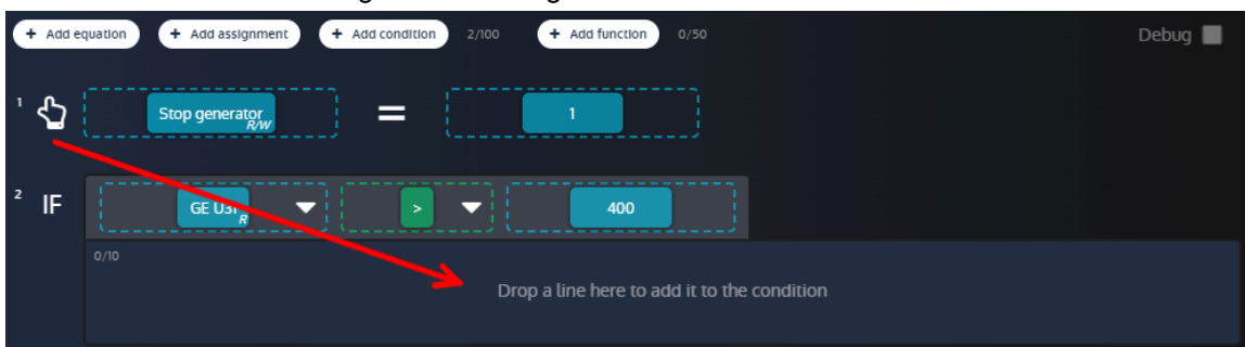
Figure 36. Adding an instruction to a condition
