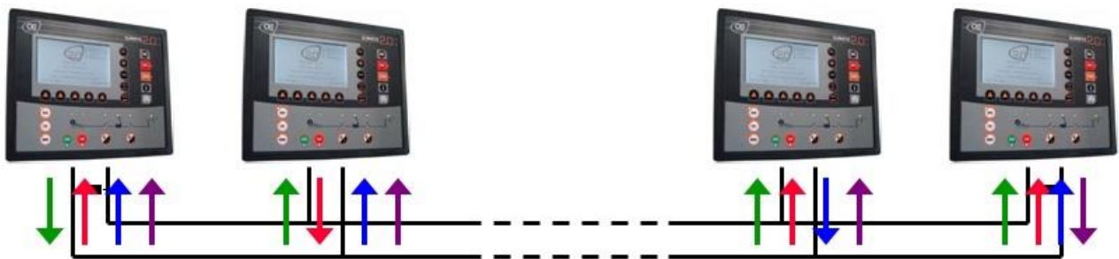
FIGURE 83 - BROADCASTING DATA BETWEEN MULTIPLE UNITS
