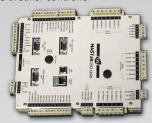
The MASTER 2.0 CORE is a controller developed to synchronize both sides of a power plant split by a bus tie breaker.
