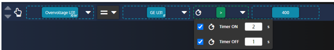
Figure 34. Setting the Timer ON/Timer OFF function of a variable block
