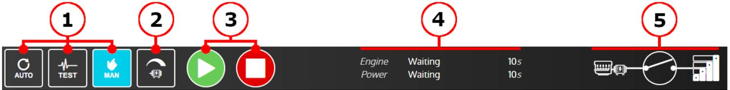
1. Controller mode buttons: Press one of this button to change controller functioning mode (auto/test/man).
