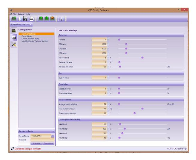
After modification, select the "Upload current page to device" icon to send displayed settings to the connected module. Select "Upload all to device" icon to send the entire configuration to the connected module.
